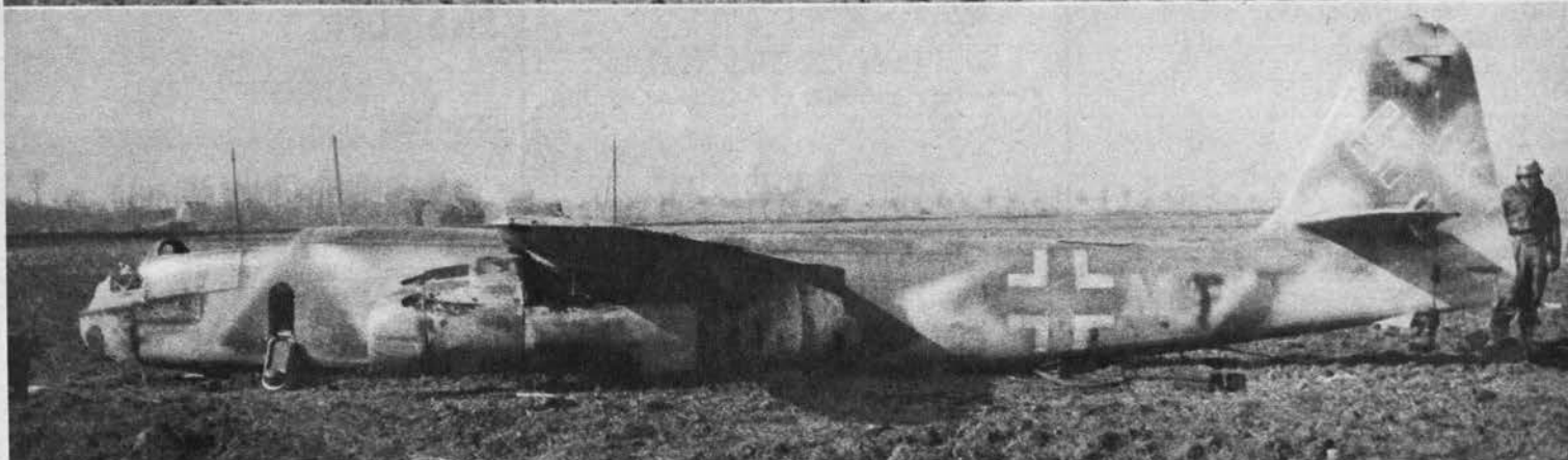
ARADO 234, NEW GERMAN JET, HAS LONG, SMOOTH LINES. NACELLES, CLEAN FUSELAGE HANG FROM HIGH WING. TAILPLANE IS TRIANGULAR
